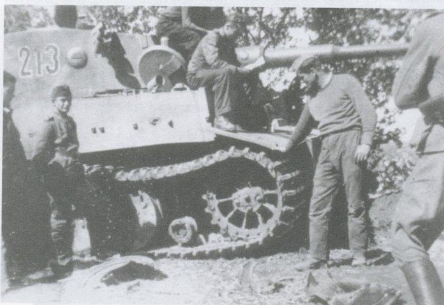
Tiger 213 has suffered additional running-gear damage through enemy fire in the area around Krasnograd, 12 September 1943.
