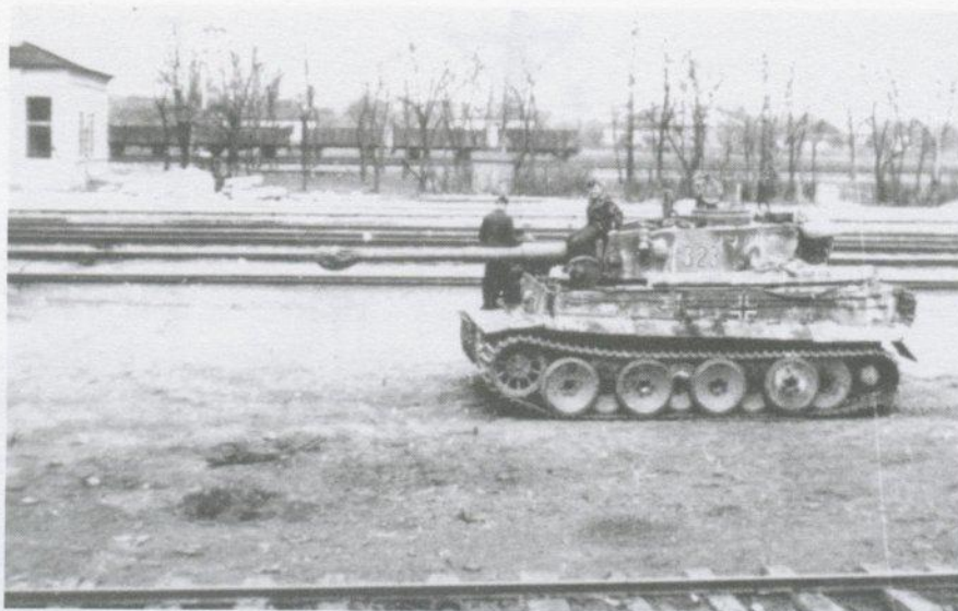
Another view of rail-loading operations at the Sartana train station in April 1943. Tiger 323 of the 3rd Company stands by to be loaded on the train. Note the narrow transportation tracks on the Tiger.
